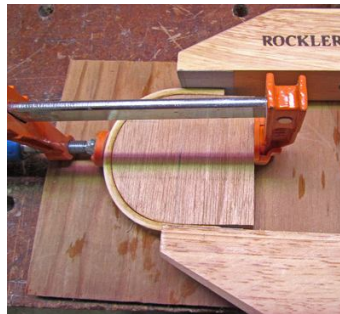
Forming the support saddles from Cold-Bend™ oak material
